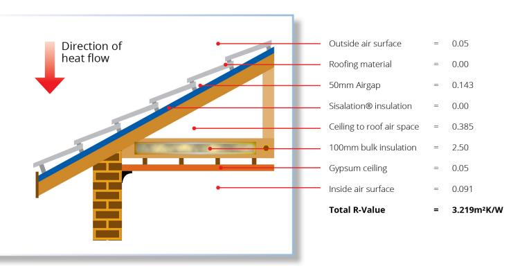
The Total R-value required is achieved by adding the R-Value of the basic elements, ie. roof and ceiling and the R-Value of any additional insulation incorporated in that element (described as the 'minimum' added R-Value of insulation'). The Total R-Value of the basic roof and ceiling has been determined by adding together the R-Values of the outdoor air film, roof cladding, roof air space, ceiling sheet lining and internal film.
